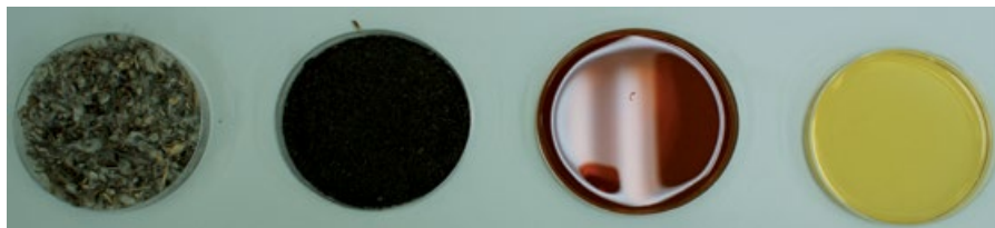
The stages in processing cotton gin trash to ethanol: raw trash; 'pretreated' or cooked trash; extracted sugars; and the fermentation beer (sugars to ethanol).
